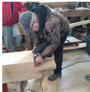
The tenon is cleaned using a belt sander by Fred Blauth..
