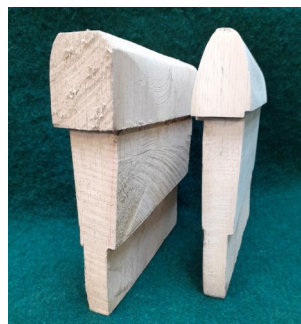
A blank on left and a finished tooth ready for use.
