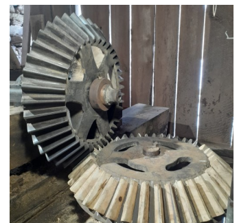
New teeth are in place in the horizontal bevel gear.
