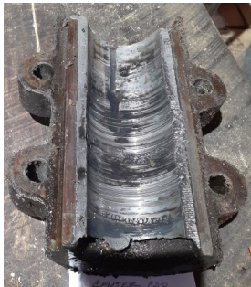
L to R—Badly worn bearing; melting old Babbitt; bearing base, cap and shaft in place, about to pour; completed bearing.
