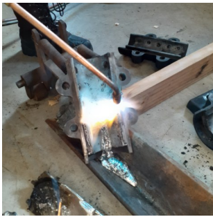
L to R—Badly worn bearing; melting old Babbitt; bearing base, cap and shaft in place, about to pour; completed bearing.
